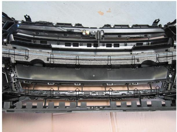
17. Undo the T30 fastener that holds the under light brace bar .
