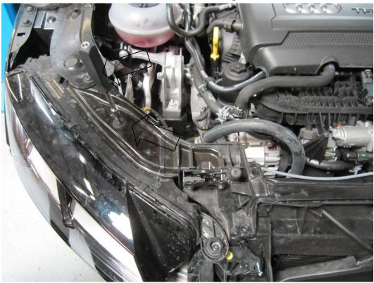
19. Disconnect the air temp sensor and remove the ducting either side of the intercooler assembly.
