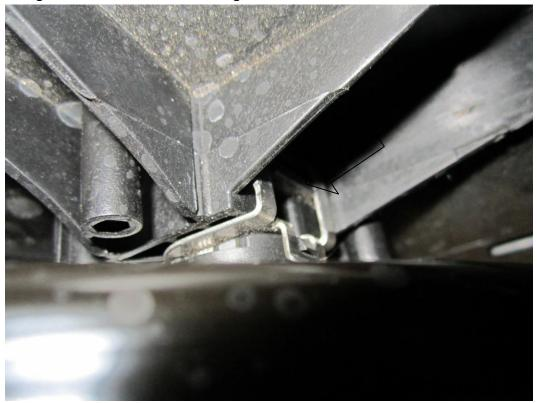
24. The light housing needs to be removed. Pull out the tab that is arrowed in the picture below then slide the housing upwards. Do not undo the bolt under the tab as this will adjust the height of your headlight.
