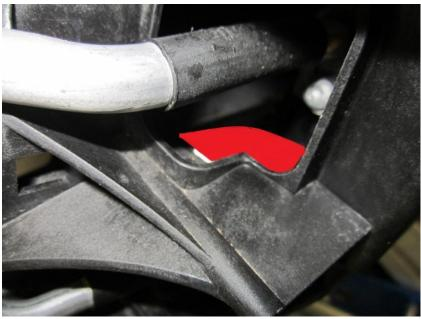
36. Once the front plastic cowl has been trimmed fit the mounting blocks to each side of the intercooler.
