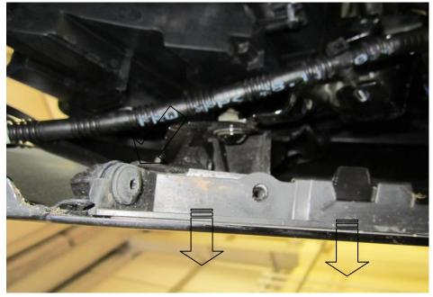
9. Disconnect the wiring loom on the inside the lower passenger side of the bumper (RHD vehicles)
