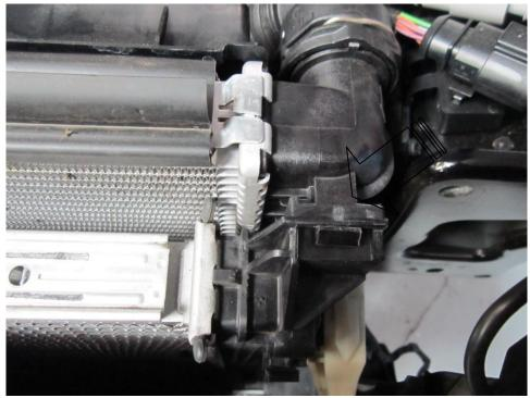
32. Remove the rubber ducting which sits either side of the condensor, This will no longer be used as your Forge Motorsport intercooler is a lot thicker than your OEM item.
