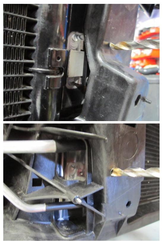
pipes can only have one of the fasteners tightened dont worry as the cowling itself will hold this in position when fully installed.
