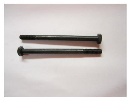
29. Using a 17mm socket remove one bolt from each side of the crash bar and replace them with the longer bolts supplied. Now remove the other 3 bolts from each side. When the jack in place the long bolts can be removed.
