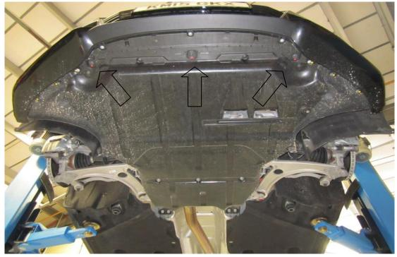
7. Now using the T20 and T45 Torx drives remove the fasteners pictured ,there are also two trim clips at the rear of the undertray that must be removed.
