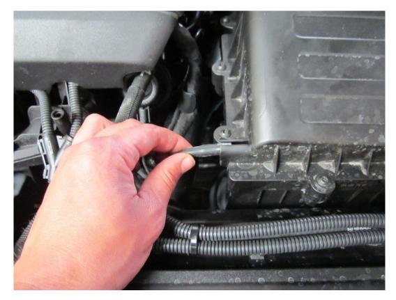
4. Loosen the clamp on the induction hose to your turbo, then pull in an upwards motion to remove.
