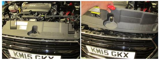
13. Remove the T20 fasteners under the plastic cover .
