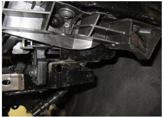
23. Next remove this tab light mechanism from the top of the headlight. Now slide the headlight out from under the housing.
