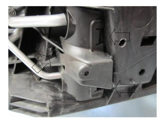
31. Pull the cowling away from you, then using a flat bladed screwdriver push down on the tabs holding the radiator to the intercooler. Push the radiator away from you while the tabs are depressed.
