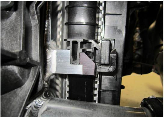
42. Before clicking the radiator into position remove the plastic cover that is mounted on top and push the radiator into the rear of the intercooler making sure the tabs are fully inserted.
