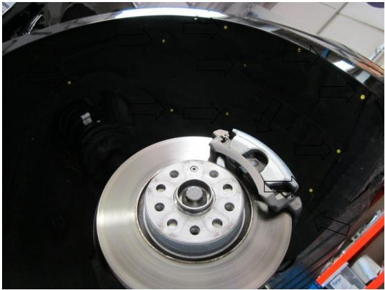
6. Using the T30 Torx drive undo the 3 fasteners pictured .
