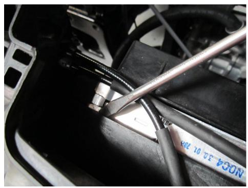
44. Now the intercooler and radiator are sat within the cowling, use the self tapping screws and penny washers provided. Insert the screws through the plastic cowling and into the mounting blocks then tighten .
