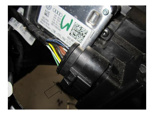
21. Undo the two T30 fasteners arrowed in the picture below.
