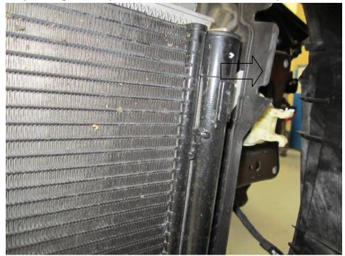
33. Push in the tabs on the top of the intercooler that hold the condensor in place then pulling or pushing the condensor in an upwards motion should remove it from the
