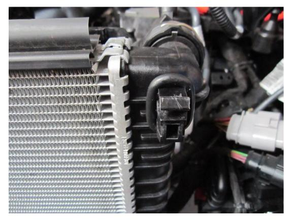
41. Place the radiator into position on the lower mounting blocks, then using a 6mm allen key, tighten into position.
