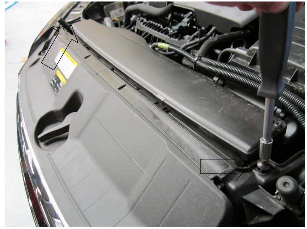
3. Remove the 6mm vac hose from the side of the airbox.
