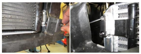
39. Please study the photos below to see where to drill the access holes in order to tighten some of the mounting clamps. The mounting clamp closest to the condensor
