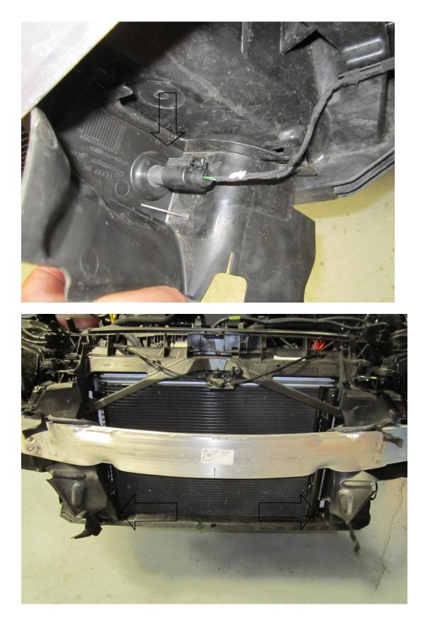
20. To remove each headlight disconnect the wiring loom on the rear of each light by pushing in the tab arrowed then pull the loom away from the headlight .
