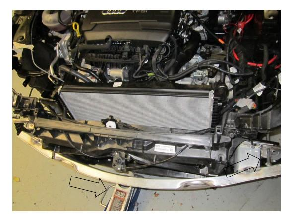
30. Remove this part of the plastic cowling where the air condensor pipes pass through the intercooler assembly housing by pushing in on the tabs as arrowed .
